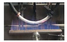
Fire Resistant designs achieve the highest rating of upto 180 minutes when subjected to integrated testing involving direct impact and high pressure water spray. The details of this test are currently documented in Annex B of BS6387, but will soon be published as a stand alone standard BS8491.
